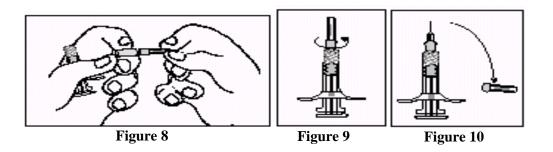
7. Hold Syringe B upright. Remove the cap on the bottom of the sterile needle cartridge by twisting it (Figure 8). Attach the needle cartridge to the end of Syringe B (Figure 9) by pushing in and turning the needle until it is firmly seated. Do not twist the needle onto the syringe until it is stripped. Pull off the clear needle cartridge cover prior to administration (Figure 10).
